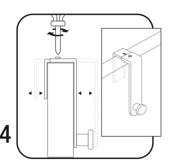
Adjust sides of the hanger to the panel/wall, screw until tight.
