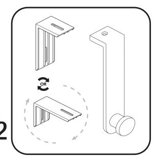
Select Bracket side according to your wall thickness. For thicker panels/walls, you will need to select the longer leg of the bracket.
