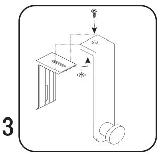
Line up the holes of the Bracket and Hanger and loosely thread the nut on the screw.
