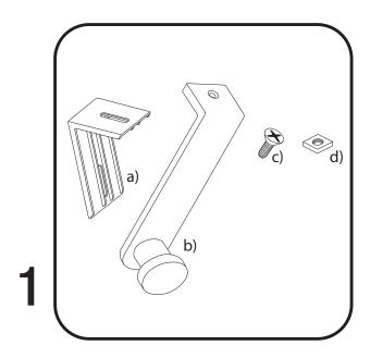
Includes: a) Bracket, b) Hanger c) Screw d) Nut
