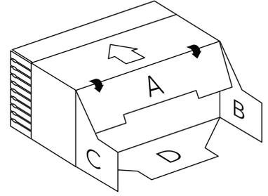
3 Fold in flaps B and C then fold up flap D and insert its tab into the slot created by flaps A, B and C.
